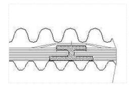
Figure 3. Low loss spacer.
